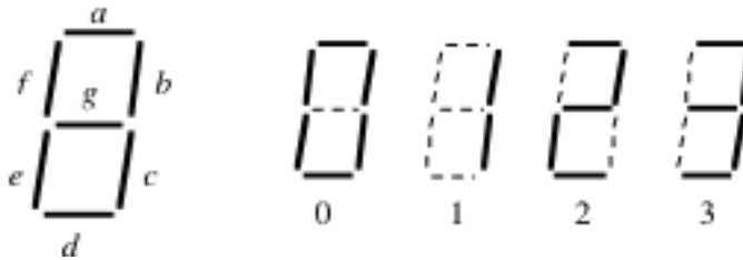
Figure 4.3.1 A single-digit seven-segment display can show 0-9 and A-F (as A, b, c, d, E, F).
