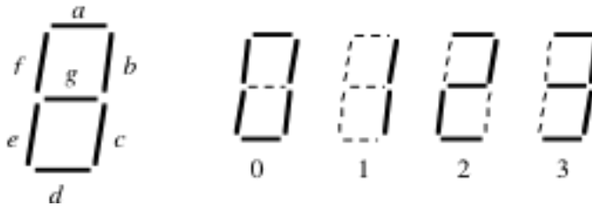
Figure 16.1.1 A single-digit seven-segment display can show 0-9 and A-F (as A, b, c, d, E, F).
